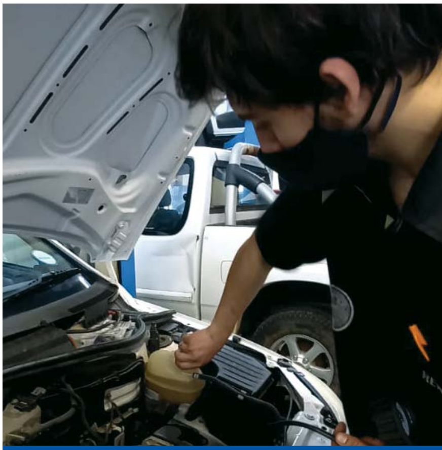
» Lombard performing pressure test on a cooling system.
