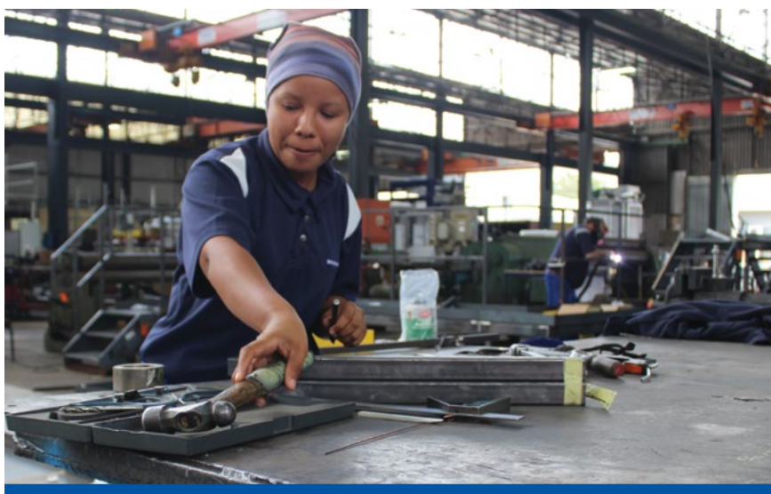
» King punching to drill a hole in the square tubing.
