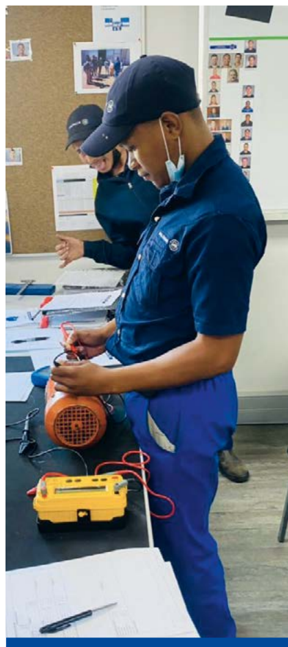
» Isolation resistance tester in use. Testing between electrical motor windings and windings and earth.
