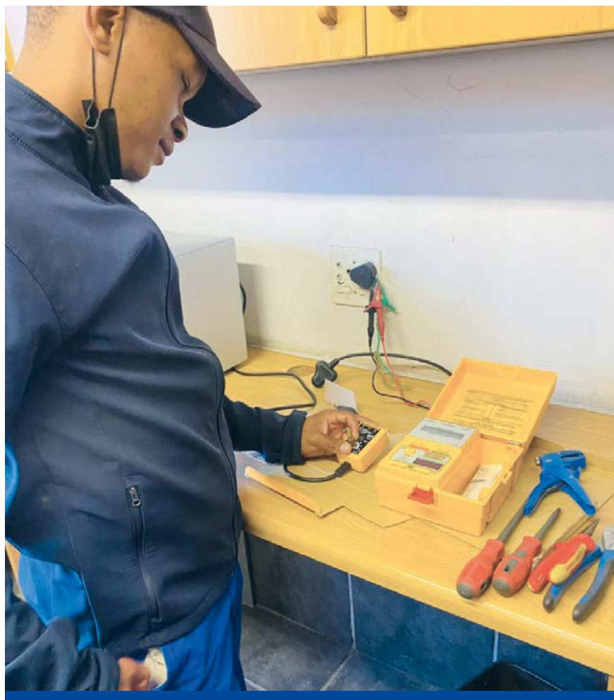
» Earth leakage tester in use for single phase plug circuit.
