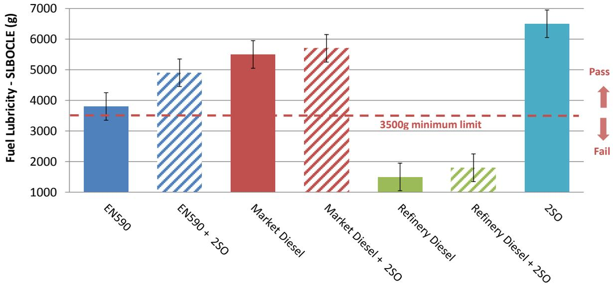
Figure 2 SLBOCLE Lubricity results
