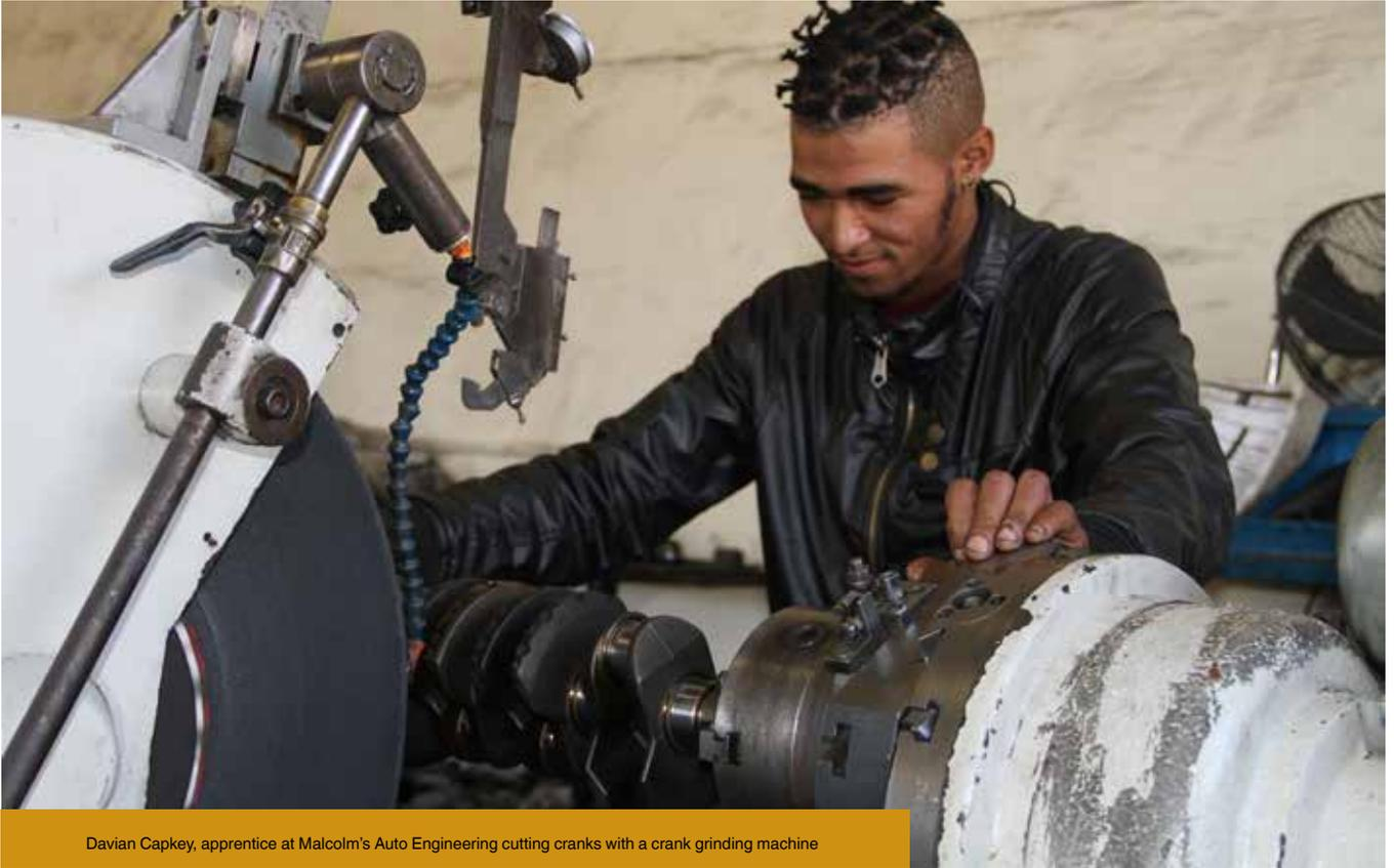
Davian Capkey, apprentice at Malcolm's Auto Engineering cutting cranks with a crank grinding machine
