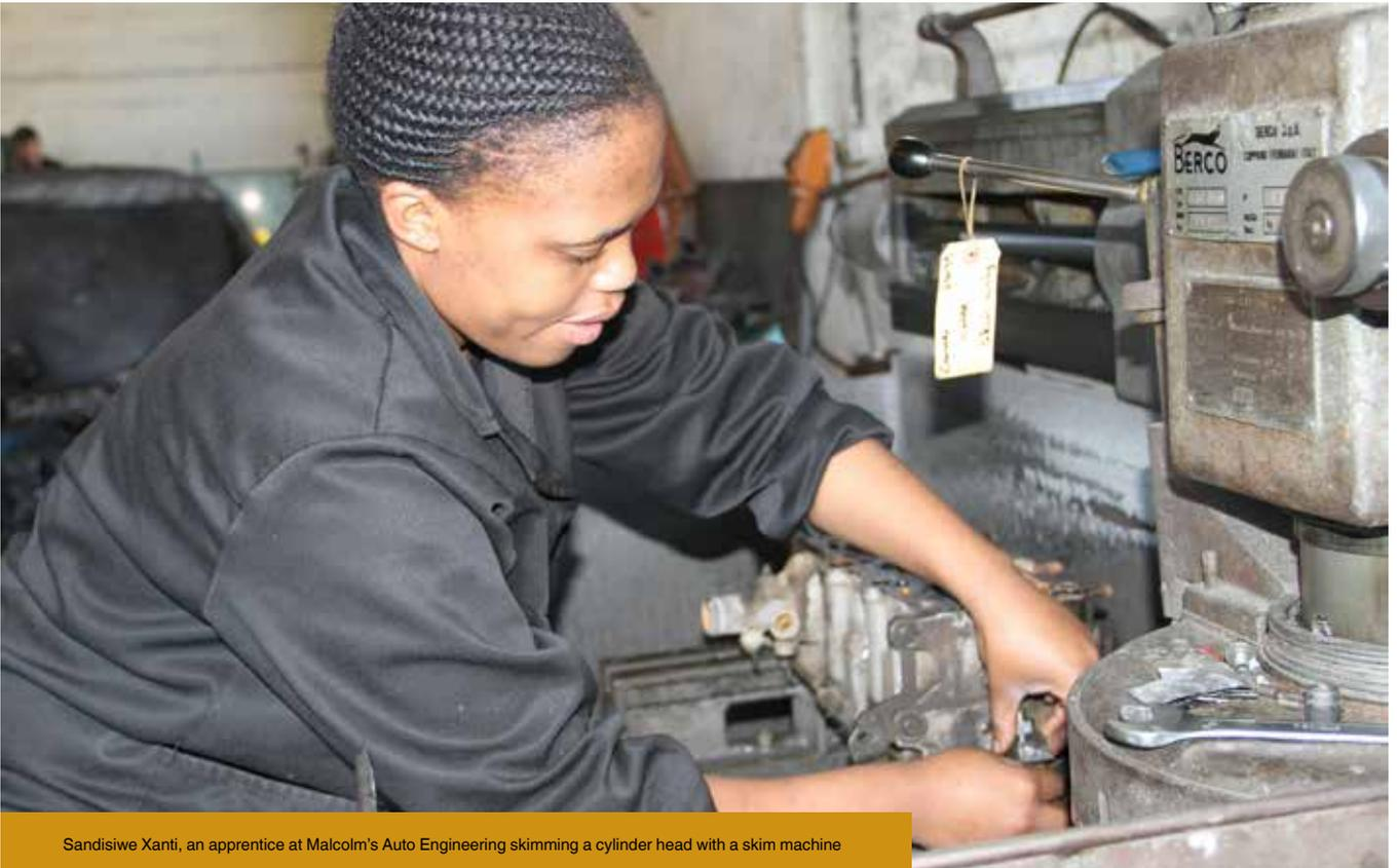
Sandisiwe Xanti, an apprentice at Malcolm's Auto Engineering skimming a cylinder head with a skim machine
