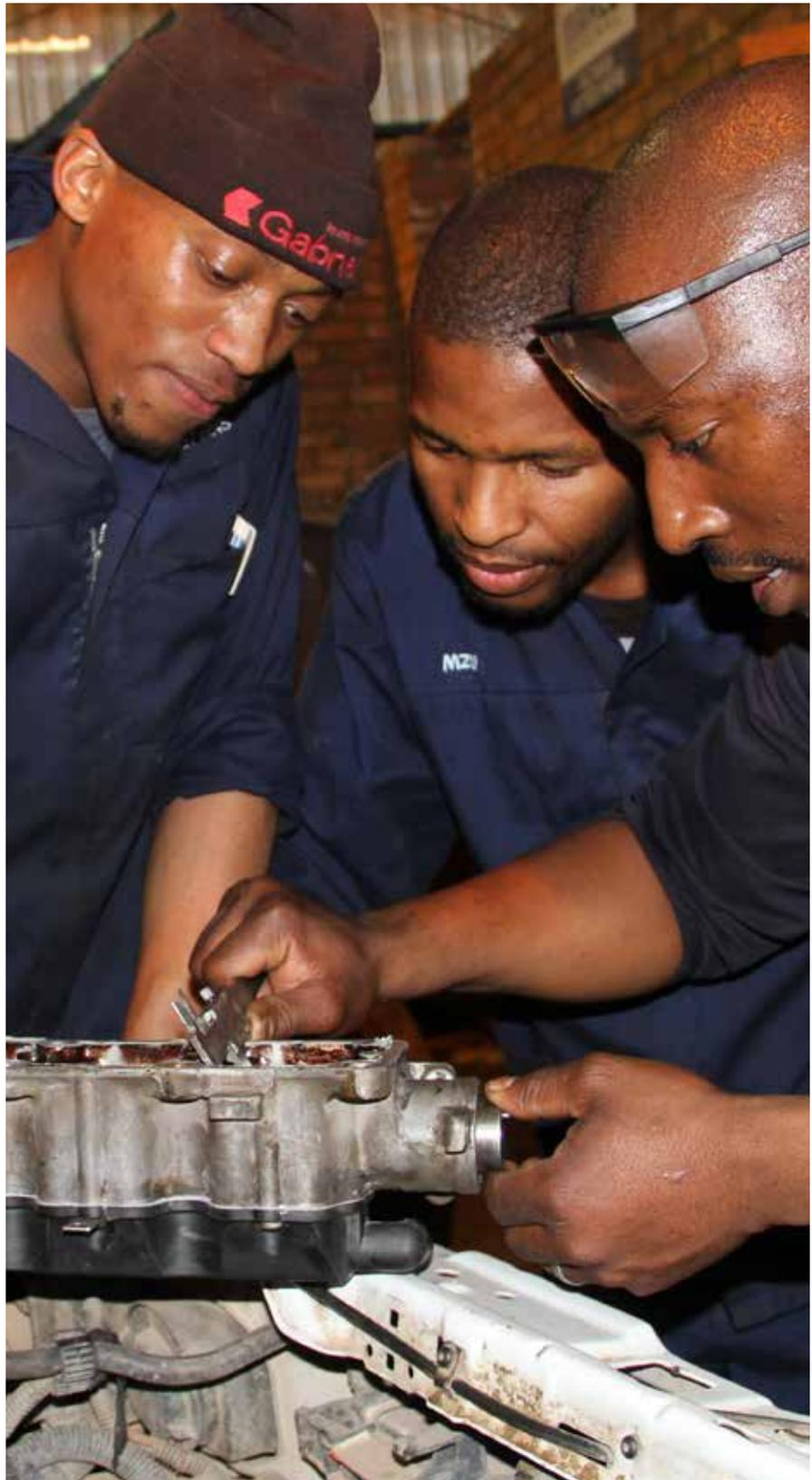
Chuma Songca with his two apprentices, Jongithemba Magadla and Mzuvelile Notshulwana checking camshaft for wear with vernier calliper on a Corsa engine
